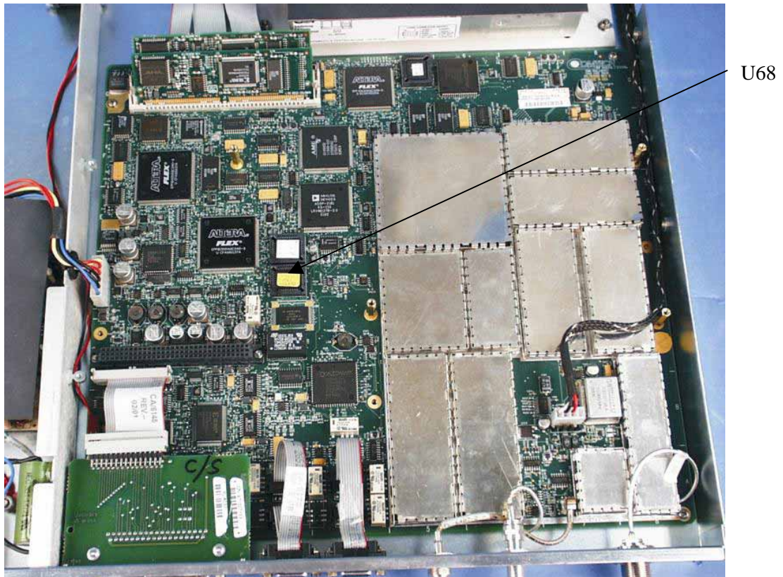
Figure 2-7. Main Board Field-Changeable Chips (Shown with Overhead Card Removed)
