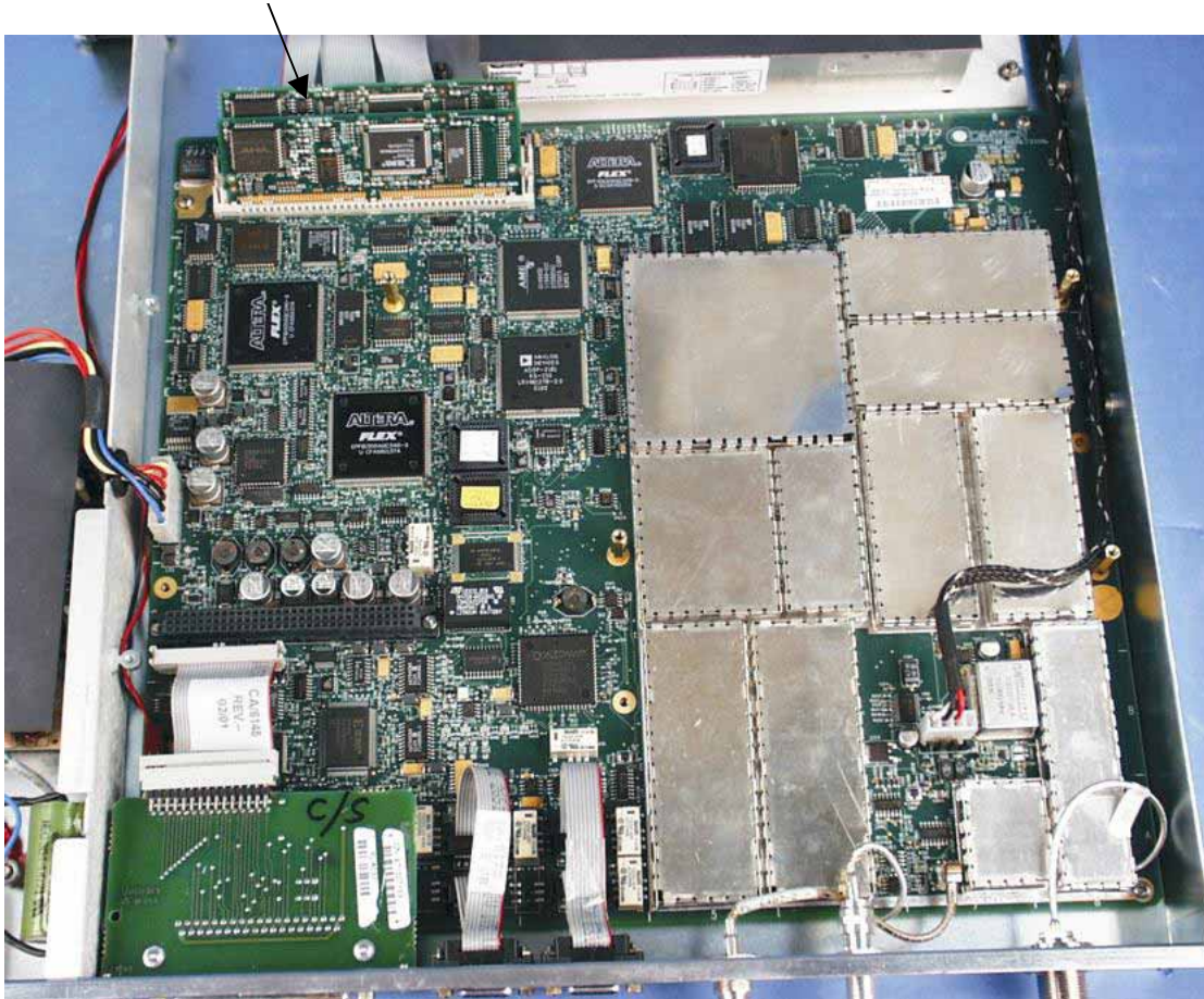
Figure 2-3. Reed-Solomon Codec Installation
